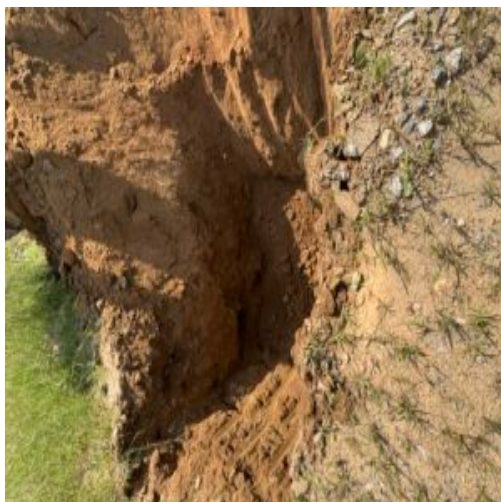
Test pits observed at onsite stockpile at Shelly Blvd.
