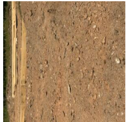
In place weathered rock materials at building lots 40 and 41. Attempted DCP tests in footings
