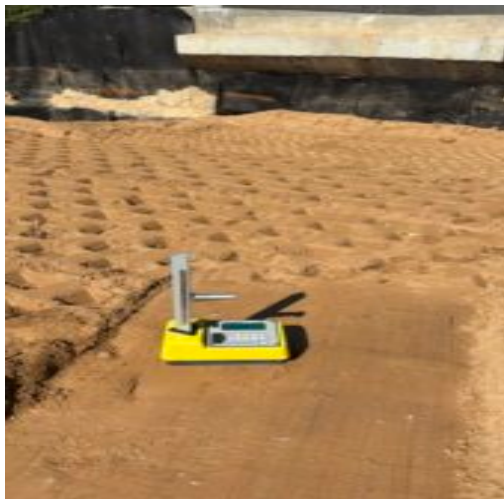
Backfill and density tests performed at west side bridge abutment
