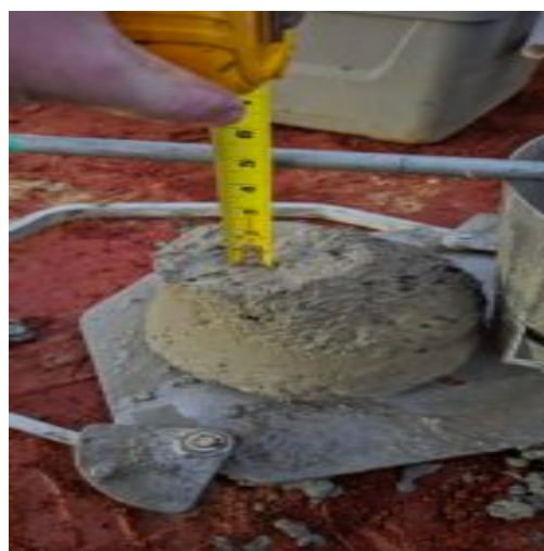
concrete slump test
