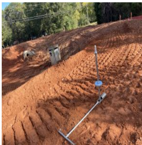
Dynamic Cone Penetrometer test at the top of the slope between Lot 19 and Pond A.
