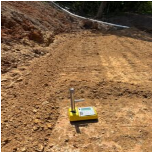
Performing density tests using Troxler Nuclear gauge
