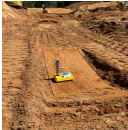
Density tests performed at sanitary sewer line between manhole #10 and 11
