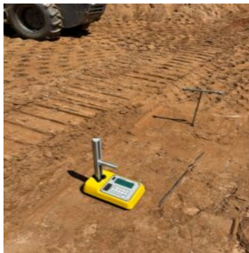
Density tests performed at sanitary sewer line between manhole #10 and 11
