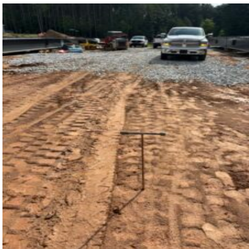
Sub grade observation at bridge approach crane pad using probe rod
