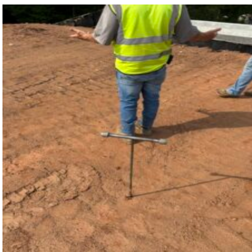
Sub grade observation at bridge approach crane pad using probe rod
