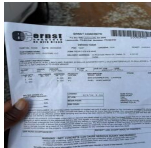
Batch ticket shows 5000 psi mix
