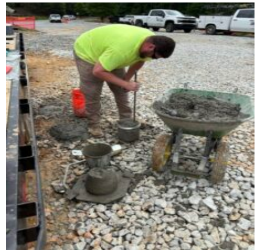
Performing air test
