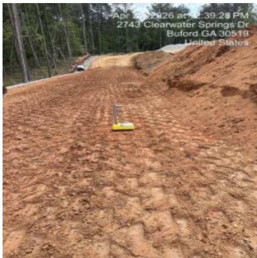
performing density testing with nuclear guage.
