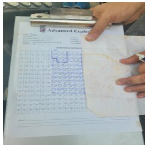
The drillers data sheet, the previous day data is covered to identify and cross check the two data sheets.
