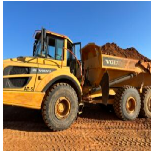
proof roll loaded tandem off road dump truck
