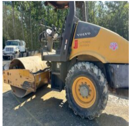
Smooth drum vibratory compactor
