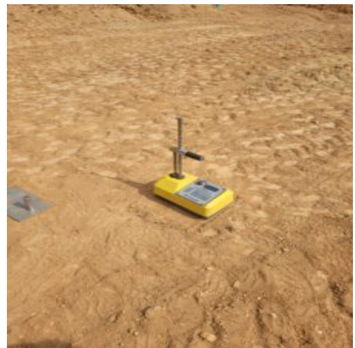
The nuclear gauge at various tests
