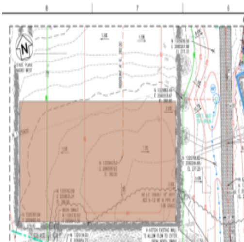
Highlighted region depicts placement of fill material section 2 part 2
